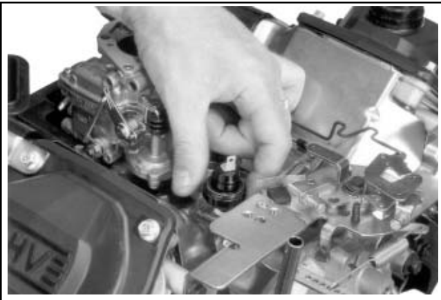
Figure 9-25. Removing Oil Sentry™ Switch from Breather Cover.
